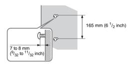
3 Peel the seals off the two screw points on the rear of the speaker.
